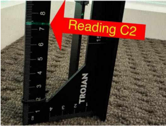
Floor level variation of approx. 27mm
